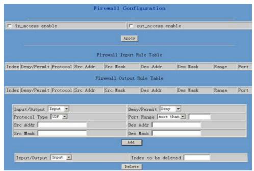
Firewall setting page. User may set up firewall to prevent unauthorized Internet users from accessing private networks connected to the Internet (input rule), or prevent unauthorized private network devices to access the internet.
