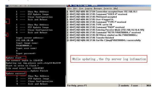
FV6020 provide safe mode. When there is booting problem because of setting problem or firmware problem. User can restore the factory setting or upgrade to a new firmware to solve this problem.
