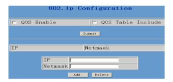
QoS Control based on 802.1p for different IP users. The QoS is used to mark the network communication priority in the data link/MAC sub-layer. FV6020 will sorted the packets using the QoS and sends it to the destination. QoS provides service classes for accessing traffics in Internet.
