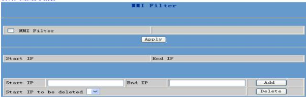
MMI filter is used to make access limit toFV6020.
