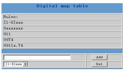
Using digital map can be combined with dial peer. First digital map will determine when the user finished dialing, then convert this number to the number actually sent according to "dial peer".
